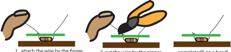
1. attach the wire by the finger (danger to jump the wire)
